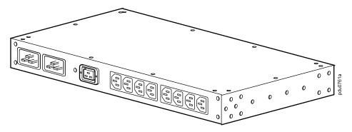
**Power inlets:** Two (2) C20 inlets support two (2) power cords (not provided) to connect the Rack ATS to two (2) separate power sources (A and B). The Rack ATS draws power from the preferred source and automatically switches to the secondary source when necessary.
