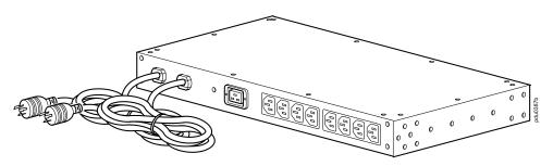
**Input power cords:** Two (2) cords connect the Rack ATS to two (2) separate power sources (A and B). The Rack ATS draws power from the preferred source and automatically switches to the secondary source when necessary. The two (2) 2.44-m (8-ft) power cords have L6-20P plugs.
