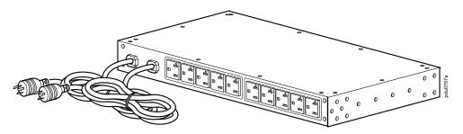
**Input power cords:** Two (2) cords connect the Rack ATS to two (2) separate power sources (A and B). The Rack ATS draws power from the preferred source and automatically switches to the secondary source when necessary. The two (2) 2.44-m (8-ft) power cords have L5-20P plugs.
