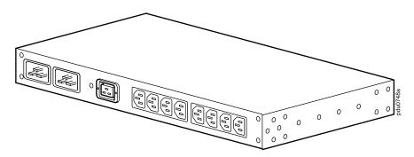
**Inlets:** Two (2) C20 inlets support the connection of two power cords (not provided) to connect the Rack ATS to two (2) separate power sources (A and B). The Rack ATS draws power from the preferred source and automatically switches to the secondary source when necessary.
