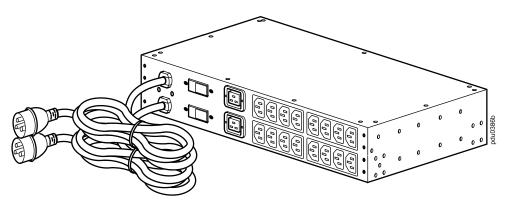
**Input power cords:** The two cords connect the Rack ATS to two separate power sources (A and B). The Rack ATS draws power from the preferred source and automatically switches to the secondary source when necessary. The two (2) 2.44-m (8-ft) power cords have IEC-309 32 A plugs.
