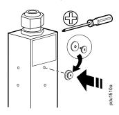
There are multiple mounting points for attaching the pegs on the back and on the side. Choose the mounting location for the pegs according to your needs.
