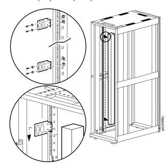
Route the power cable out of the rack and connect it to an appropriately rated branch circuit of your power source. The Rack PDU should be connected to a dedicated branch circuit protected by an appropriately sized circuit breaker. Turn the power feed circuit breaker ON, only after the connection to the Rack PDU is complete.
