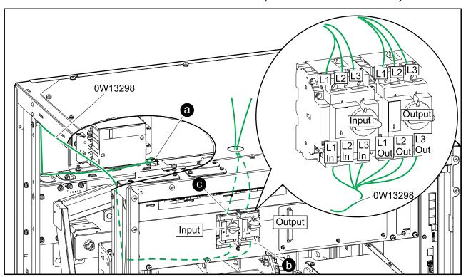
NOTE: Minimum power cable size is 2.5 mm<sup>2</sup> (14 AWG).
