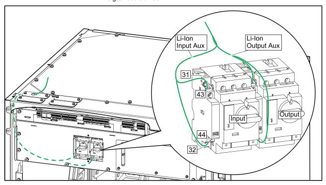
7. Reinstall the plate and install the two protection covers over the battery control breakers.
