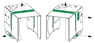
5. Install the backfeed kit frame and the two plastic box pieces. Connect the small bracket from the backfeed kit frame to the corner pillar of the UPS. Use the provided M6x16 screws and M6 nuts.
