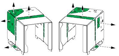
5. Install the backfeed kit frame and the two plastic box pieces. Connect the small bracket from the backfeed kit frame to the corner pillar of the UPS. Use the provided M6x16 screws and M6 nuts.
