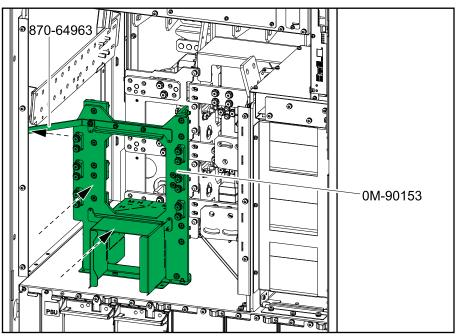
6. Install the six backfeed kit busbars and the three input busbars on the backfeed kit frame and connect to the busbars in the UPS. The input busbars were removed from the UPS in step 3.
