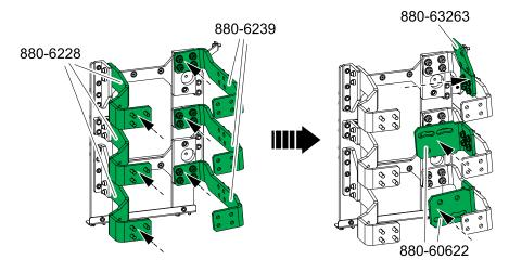
7. Follow the UPS installation manual to connect the power cables. Note that the input busbars are now located on the backfeed kit assembly.
