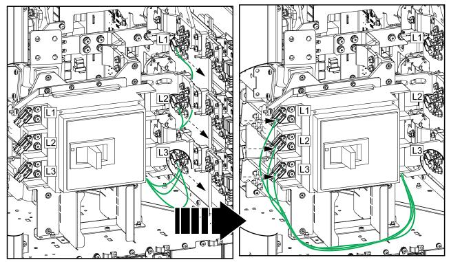
10. Remove the system level controller and disconnect the preconnected signal cables 0W13234 and 0W13276 from board 0P4828.
