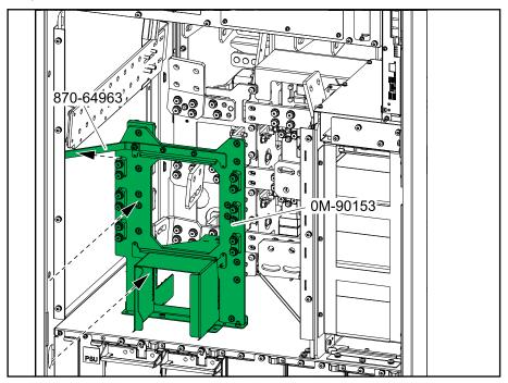
6. Install the three backfeed kit busbars and the three bypass busbars on the backfeed kit frame and connect to the busbars in the UPS. The bypass busbars were removed from the UPS in step 3.
