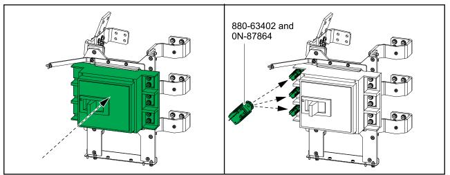
9. Disconnect the preconnected signal cables from the measurement boards on the side of the static bypass switch. Connect the signal cables to the new service measurement boards on the backfeed breaker. The signal cables will make a click when connected properly.
