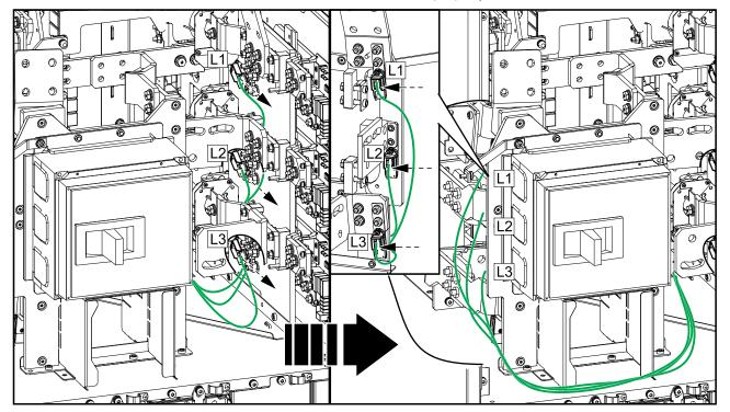
9. Remove the system level controller and disconnect the preconnected signal cables 0W13234 and 0W13276 from board 0P4828.
