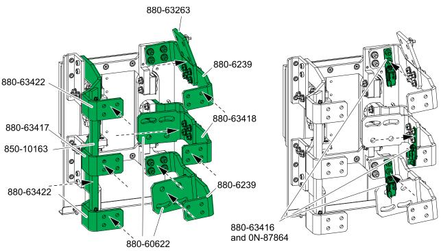
7. Follow the UPS installation manual to connect the power cables. Note that the input busbars are now located on the backfeed kit assembly.
