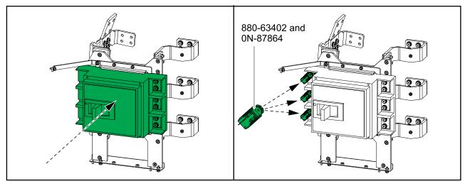
9. Disconnect the preconnected signal cables from the measurement boards on the side of the static bypass switch. Connect the signal cables to the new service measurement boards on the backfeed breaker. The signal cables will make a click when connected properly.
