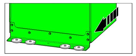
3. Lower the levelling feet until they connect with the floor - use a bubble-leveler to ensure that the cabinet is level.
