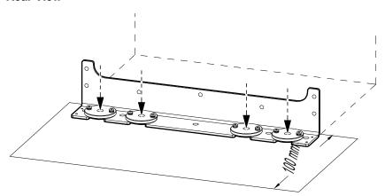
2. In systems with more battery cabinets, interconnect the seismic assemblies with the interconnection plate 870-51172 from the accessory kit 0M-95331.
