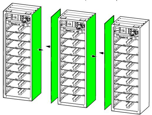
2. Push the right-most battery cabinet into position. For seismic anchoring, ensure that the rear seismic bracket connects to the rear anchors.
