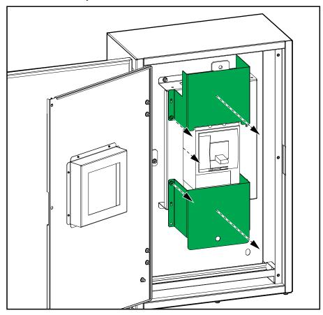
3. Remove the cover on the battery breaker.
