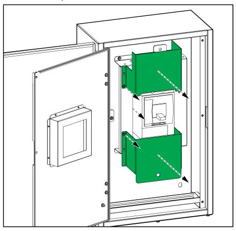
3. Remove the cover on the battery breaker.
