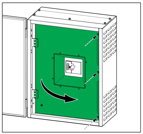
15. Close and lock the front door of the battery breaker box.
