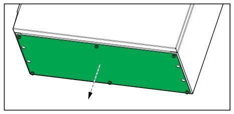
2. Drill or punch holes for cables or grommets in the gland plate.
