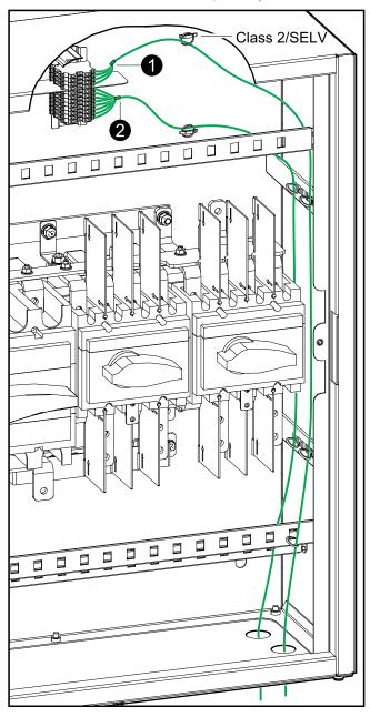
1. Connect the Class 2/SELV signal cables for the breaker indicator lights from the control terminal block in the maintenance bypass panel to the UPS as per your configuration.
