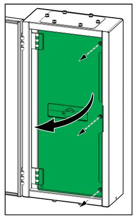
4. Mount the output switch box to the wall.
