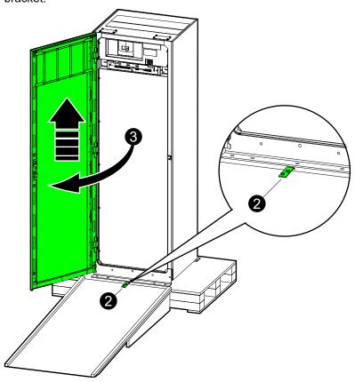
5. Remove the front and rear shipping brackets.
