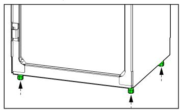
7. Roll the battery cabinet carefully down the ramp.
