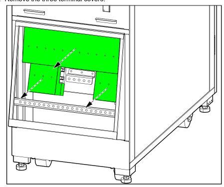
Connect the Power Cables 10-40 kVA 208 V UL
