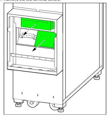
10-40 kVA 208 V UL Connect the Power Cables
