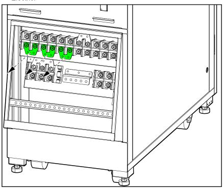
5. Remove the gland plate from the bottom of the conduit box. Drill or cut holes in the gland plate for cables/conduits. Install conduits (if applicable) and reinstall the gland plate.
