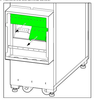
Connect the Power Cables 10-40 kVA 208 V UL
