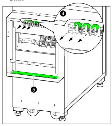
Remove the gland plate from the bottom of the conduit box. Drill or cut holes in the gland plate for cables/conduits. Install conduits (if applicable) and reinstall the gland plate.
