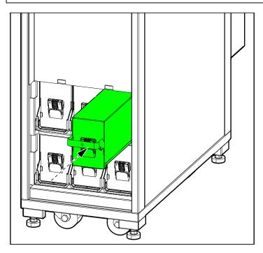
5. Push down the handle and fasten the battery module with a screw in front of the battery module.
