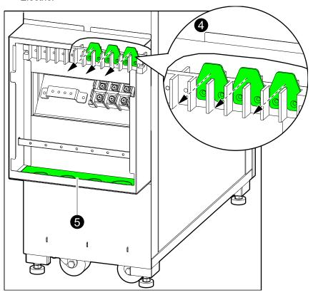
5. Remove the gland plate from the bottom of the conduit box. Drill or cut holes in the gland plate for cables/conduits. Install conduits (if applicable) and reinstall the gland plate.
