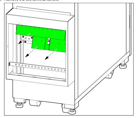
10-40 kVA 208 V UL Connect the Power Cables
