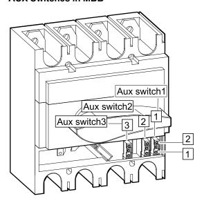
Connect the signal cables (not supplied) from the three AUX switches in the MBB to the UPSs.
