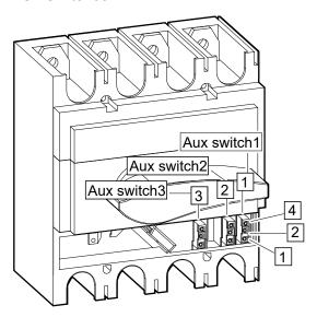
**NOTE:** UOB contains one AUX switch and MBB contains three AUX switches.
