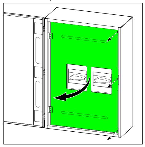
2. Drill holes in the four marked locations in the wall and mount the anchor bolts.
