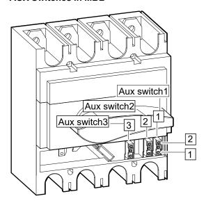
2. Connect the signal cables (not supplied) from the three AUX switches in the MBB to the UPSs using one of the following methods.
