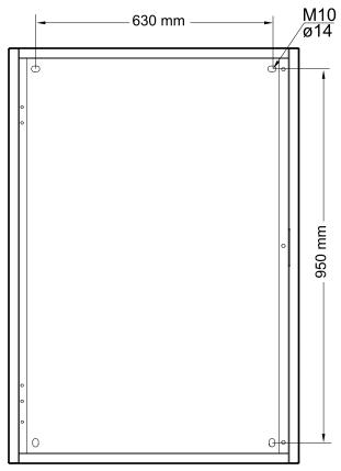
3. Mount the maintenance bypass panel to the wall.
