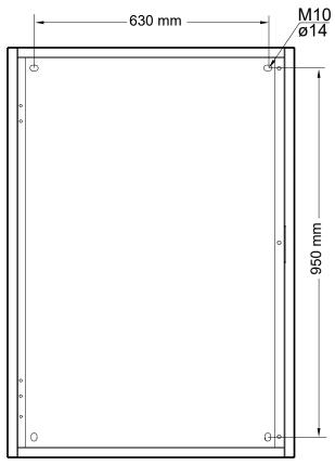
3. Mount the maintenance bypass panel to the wall.
