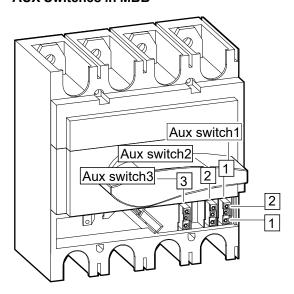
2. Connect the signal cables (not supplied) from the three AUX switches in the MBB to the UPSs.
