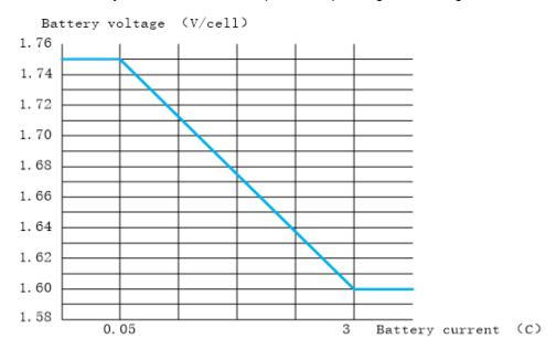
The Low Battery Shutdown level is 1.61 to 1.74 per cell depending on discharge ratio.
