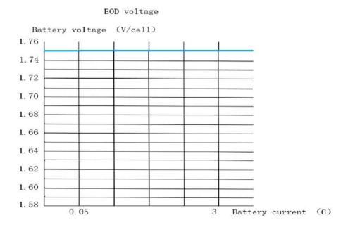
The Low Battery Shutdown level is 1.76 to 1.8 per cell depending on discharge ratio.
