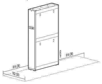
The free space on the rear part of the unit is needed for moving the equipment and the free space on the front part of the unit is needed to grant service access, whenever the equipment is located in a row.
