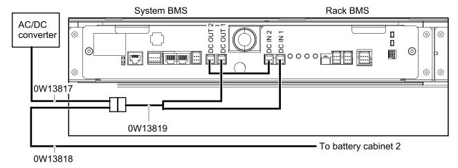
4. **In battery cabinet 1**: Connect the provided cable 0W13819 to port DC OUT 1 and port DC IN 1 in the SMPS/BMS box as shown above.
