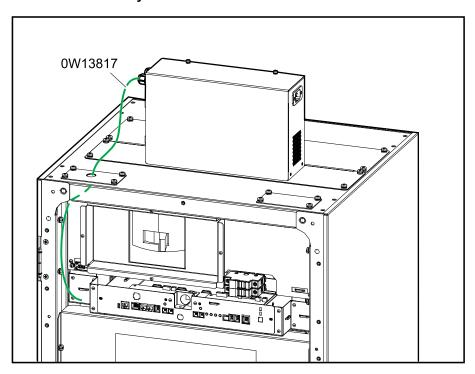
3. **In battery cabinet 1**: Connect cable 0W13817 to the connector on the provided cable 0W13819 pin 1 and pin 2.
