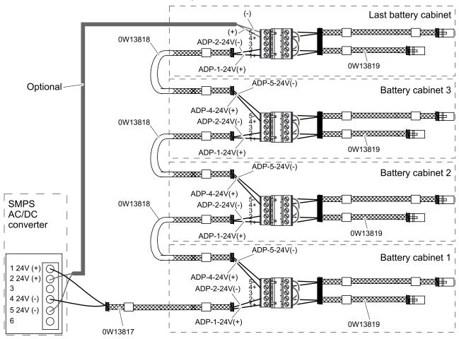
6. **In battery cabinet 2**: Connect cable 0W13818 to the provided cable 0W13819 with the connector on pin 1 and pin 2.
