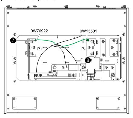
8. Disconnect the internal cable 0W13501 from the P- busbar. Reinstall the nut on the P- busbar.
