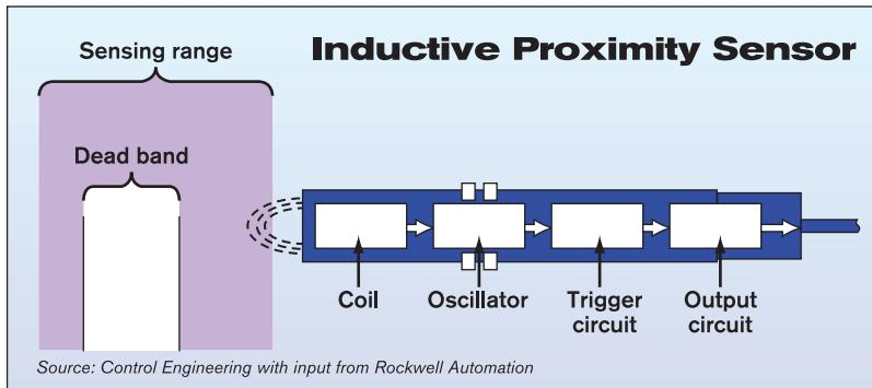
An inductive proximity sensor contains a coil to generate an electromagnetic field, an oscillator circuit to excite the coil, a trigger circuit, and an output circuit. The latest sensors can be programmed to sense an object at defined places within the field rather than just anywhere within the field.
