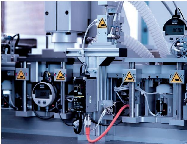
*Flexible fiber-optic cabling from a DIN-rail mounted amplifier allows technicians to detect an object deep in a machine while allowing access to the sensor as shown in this application photo from Omron.*
