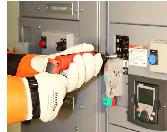
Electric screwdriver (10 mm hex with 10N-m torque)
