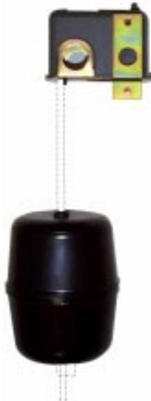
The Class 9036 Type FG 31 float switch is designed for liquid level control with electric motor operated pumps either directly or through a magnetic starter. It can also be used to activate alarms in liquid level control systems. The upward or downward movement of the lever arm of the Class 9036 Type FG 31 float switch controls the ON and OFF positions corresponding to the water levels changes required to turn the pump or alarm on and off.
