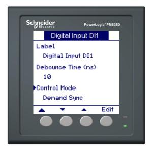
When using a digital input for demand sync, the selected demand method must be "Input Synchronized Block," or "Input Synchronized Rolling Block," and the demand interval duration and demand subinterval duration configurations must be the expected durations. The demand sync pulse from the external meter must occur within +/- 5 seconds of the expected duration to be considered a valid sync pulse.
