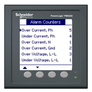
If you make changes to the basic power meter setup, all alarms are disabled to prevent undesired alarm operation. Confirm alarm configuration and enable required alarms.
