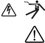
The addition of either symbol to a “Danger” or “Warning” safety label indicates that an electrical hazard exists which will result in personal injury if the instructions are not followed.
