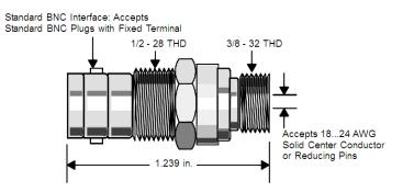
The 52-0370-000 Self-terminating BNC Adapter has a return loss of 40 dB, a frequency range from 100 kHz ... 30 MHz, and an insertion loss of 0.03 dB.
