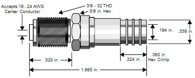
A Modicon 52-0399-000 model for non-quad shield cable
