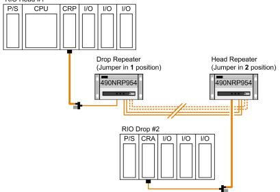
In an optical bus connection, one repeater is always the drop and all other repeaters are heads: RIO Head #1
