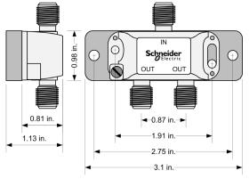
**NOTE:** When not in use, splitter ports must be terminated with a Modicon 52-0402-000 Port Terminator.
