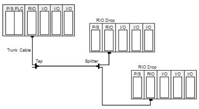
**NOTE:** Branching is permissible when fiber optic cable is used. See *Using Fiber Optics in an RIO System, page 33.*
