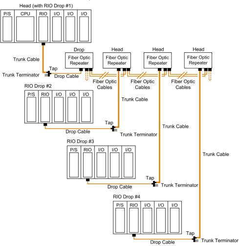
Five chained 490NRP954 fiber optic repeater can be linked in a bus topology. This number can be reduced by the total pulse width distortion (jitter) that occurs on the system *(see page 59)*. Twelve chained 140NRP95400 fiber optic repeater can be linked in a bus topology. Twelve chained 140NRP95401C fiber optic repeater can be linked in a bus topology.
