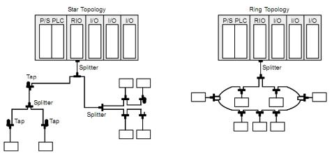
**NOTE:** These kinds of topologies are also not permissible when fiber optic cable is used. See *Using Fiber Optics in an RIO System, page 33.*
