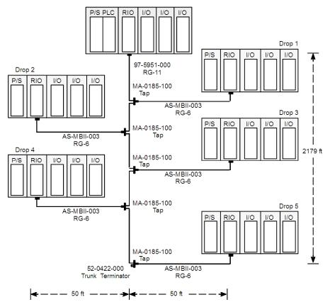
This system uses RG-11 cable for the trunk; for illustration purposes, its specified attenuation is 0.24 dB/100 ft at 1.544 MHz. Running to the adapter at drop 5 is a Modicon AS-MBII-003 RG-6 drop cable, a 50 ft cable with an attenuation of 0.3 dB. To calculate end-to-end attenuation on the trunk cable (TCA), multiply 0.24 dB (the trunk attenuation per 100 ft) by 21.79:
