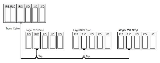
All remote drops on an RIO network must be connected to a trunk cable via a tap and a drop cable, and the last tap on a trunk cable must be terminated with a 75  $\Omega$  Modicon 52-0422-000 Trunk Terminator.
