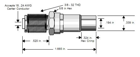
Both of these self-terminating F adapters have a return loss of 22 dB, a frequency range from 100 kHz ... 30 MHz, and an insertion loss of 0.03 dB.
