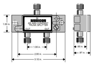
Schneider Electric MA-0186-100 (PV:01) Splitter dimensions:
