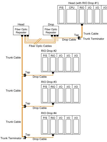
The distance between the two repeaters is limited by the maximum allowable attenuation of the fiber optic cable used in the installation. Fiber attenuation is calculated separately *(see page 57)* from coaxial cable attenuation.
