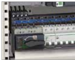
Linergy FM device feeder 80 A. The Linergy FM device feeder snaps easily onto the back of the rails. All types of modular devices can be mixed in the same row and phase balancing is simple. It's easy to change or add devices.
