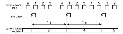
As shown in the figure, the counter current value represents the number of events accumulated during the previous 1 s interval (time base). That is, the count of the last event from IN A (n) is reported as output to the current value register (see p.~100) while events in the next 1 s interval are counted. After the four events in that interval are counted, a 4 is placed in the current value while events in the next interval are counted.
