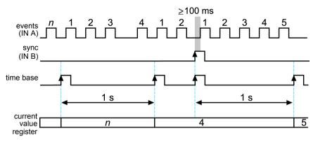
In the above figure, notice how the sync pulse can establish an interval between counting operations. The events that occur during that interval are not accumulated in the current value.
