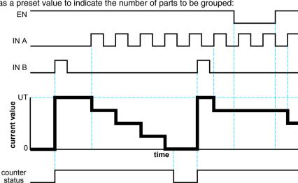
The one-shot counting mode uses the user-configured upper threshold (UT) value as a preset value to indicate the number of parts to be grouped:
