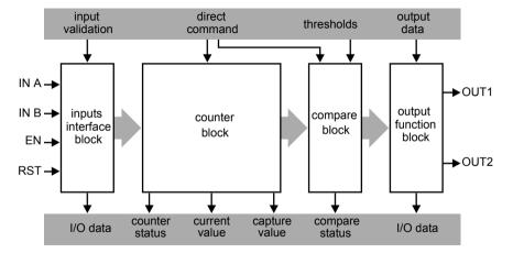
The module's onboard counter uses up to four digital inputs to produce a 16-bit *current value* result.
