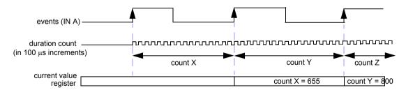
As shown above, the duration in edge-to-edge mode is measured from the rising edge of one event to the rising edge of the next event.
