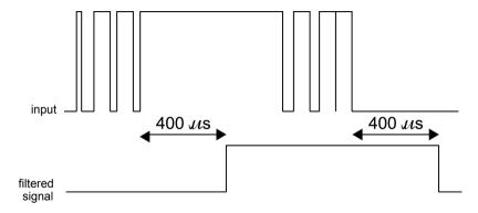
As the figure shows, the filtered signal is not on until the input has been consistently high for the configured time (400  $\mu$ s). Likewise, the filtered signal is off when the input is consistently low for the configured time.
