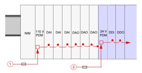
Each basic PDM contains on 5 A time-lag fuse that protects the I/O modules in the segment. This fuse is user-replaceable.
