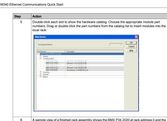
A sample view of a finished rack assembly shows the BMX P34 2020 at rack address 0 and the BMX NOE 0100 at address 1:
