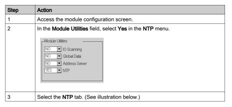
The figure shows the NTP dialog box for BMX NOE 01x0 modules:
