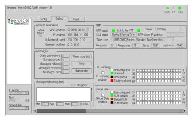
**NOTE:** The debug screen dynamically updates the Ethernet module's communication services (I/O scanning, global data, etc.).
