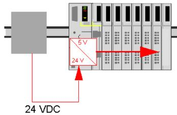
The figure below shows how the 24 VDC signal is distributed to an extension segment across the island:
