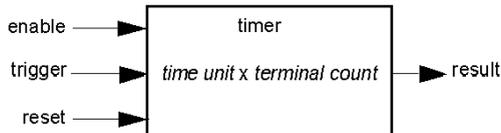
The trigger input starts the timer at 0 and accumulates *time units* of 1, 10, 100 or 1000 ms for a specified number of counts. The reset input causes the timer accumulator to be reset.
