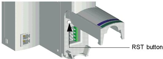
Holding down the RST button for 2 seconds or longer causes Flash memory to be overwritten, resulting in a new configuration for the island.
