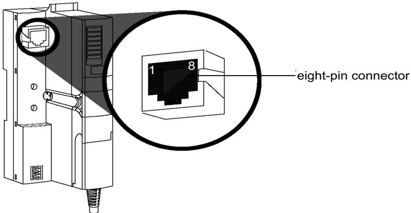
The RJ-45 connector is an eight-pin female connector. The eight pins connect horizontally along the top. Pin 8 has the leftmost position, and pin 1 is the rightmost. The pin-out for the RJ-45 complies with the information in the following table:
