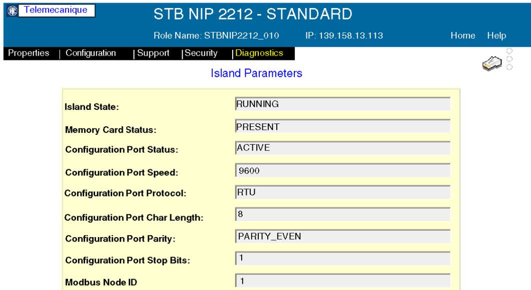
The screenshot shows a web interface for 'STB NIP 2212 - STANDARD'. The header includes 'Telemecanique' and 'Role Name: STBNIP2212\_010 IP: 139.158.13.113'. A navigation bar contains 'Properties', 'Configuration', 'Support', 'Security', and 'Diagnostics'. The main content area is titled 'Island Parameters' and displays a table of parameters:
