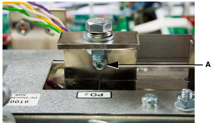
Figure 178: Bus Bar Connection Detail
