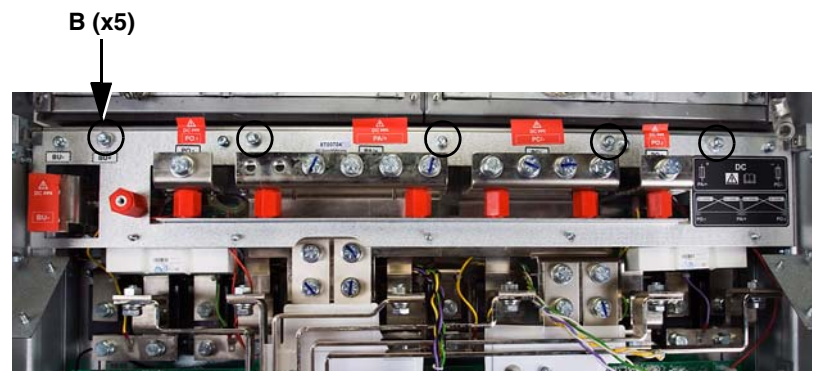
Figure 37: Top Terminal Bracket Mounting Hardware
