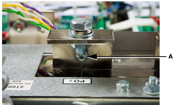
Figure 70: Bus Bar Connection Detail
