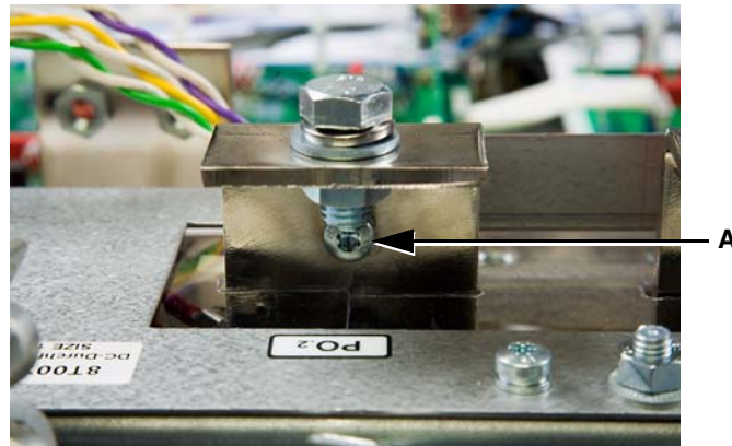
Figure 37: Top Terminal Bracket Mounting Hardware
