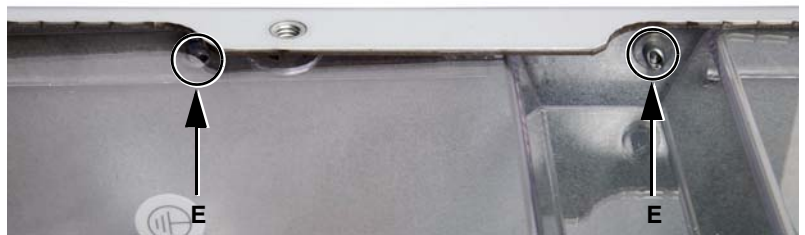
Figure 48: Terminal Shield Retaining Posts
