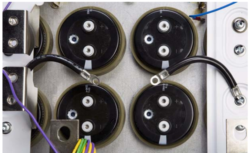
Figure 72: Capacitors, Phase V Shown
