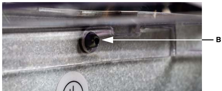
Figure 24: Power Terminal Shield Retaining Post
