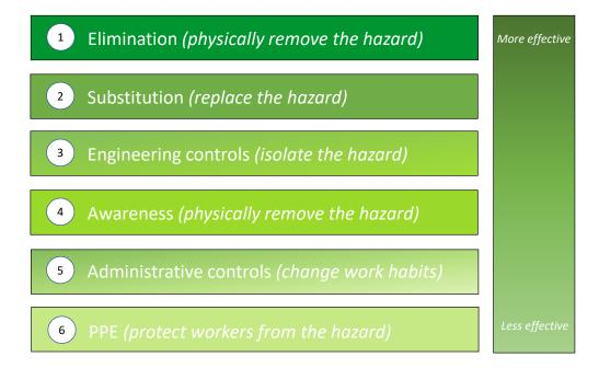
Figure 2 Hierarchy of arc flash mitigation controls
