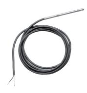
The STD550 is intended for measuring air temperature in fan coil applications or exhaust ducts. The sensor, which is made of stainless steel, is delivered with a 2 m (6.5 ft.) cable PVC sheathed overall. Mounting details such as screw and clamp are included on delivery.
