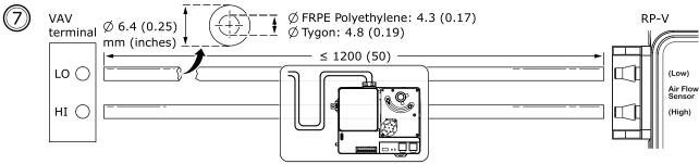
NOTE: When operating in an unusually dusty environment, connect an in-line air filter (Schneider Electric part number 01-2100-272 or equivalent filter) on the high side pressure tube from the VAV box with the filter positioned close to the VAV box. The filter helps prevent dust from entering the velocity measurement tube.
