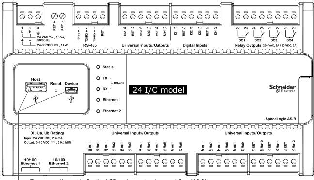
The connection cable for the USB ports must not exceed 3 m (10 ft).
