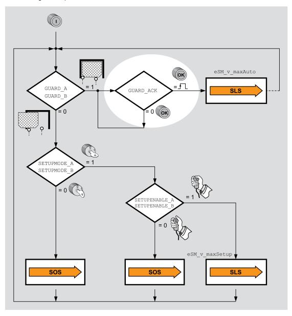
If the use of an acknowledge/reset pushbutton has been parameterized, the acknowledge/reset pushbutton must be pressed before a movement can be started in the machine operating mode Automatic Mode after the guard door has been closed.
