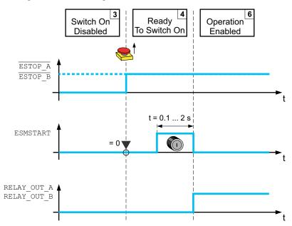
The safety module eSM monitors the duration of the start/restart pulse at the input *ESMSTART* in order to detect contact welding at the start/restart pushbutton.
