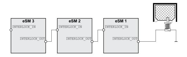
By connecting the output *INTERLOCK\_OUT* of a safety module eSM to the input *INTERLOCK\_IN* of the next safety module eSM, you can chain signals, for example, for a multi-axis system.
