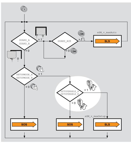
If the enabling switch is not activated, the safety-related function SOS is active in machine operating mode Setup Mode when the guard door is open.
