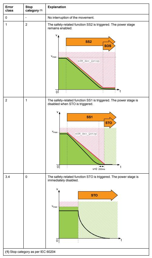
Errors of classes 0, 1, 2, and 3 are reset with the function "Fault Reset" of the drive after the cause of the detected error has been removed. Errors of class 4 can only be reset with a power cycle of the drive. Refer to the user guide of the drive for details.
