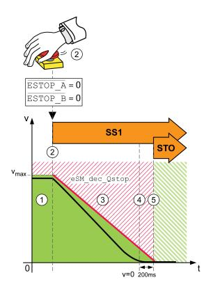
The following steps are performed in the case of an Emergency Stop:
