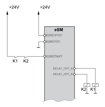
The start/restart signal is available at the inputs *ESMSTART* of the safety modules eSM for a period of 100 ms. During this time the connected safety modules eSM must recognize the start signal. When this time has passed, the two power contactors at the outputs *RELAY\_A* and *RELAY\_B* switch. The normally closed contacts interrupt the start/restart signal.
