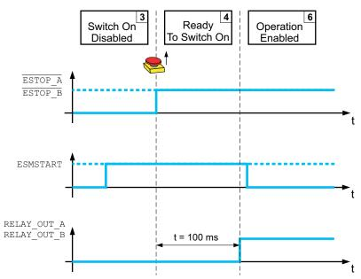
If automatic start/restart is configured, the safety module eSM verifies that the level at the input *ESMSTART* is 1.
