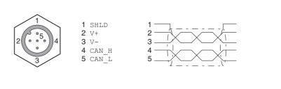
Figure 6.10 Pin assignment industrial connector
