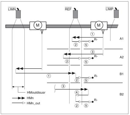
Figure 8.14 Reference movements to the reference switch
