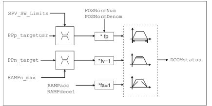
Figure 8.10 Operating mode Profile Position, effect of adjustable parameters
