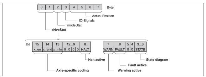
Figure 8.2 Structure of driveStat
