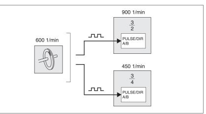
Figure 8.7 Reference value via NC controller
