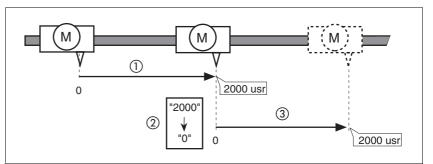
Figure 8.19 Positioning by 4000 usr units with position setting
