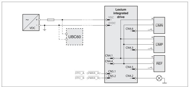
Figure 6.1 Wiring example
