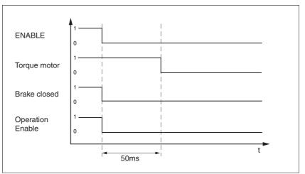
Figure 8.30 Applying the holding brake
