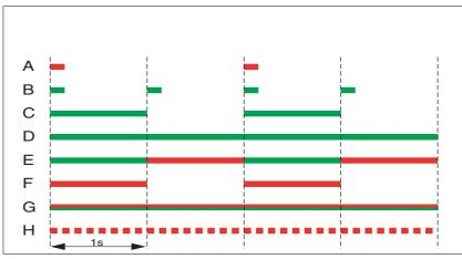
Figure 10.2 Error indication with LEDs
