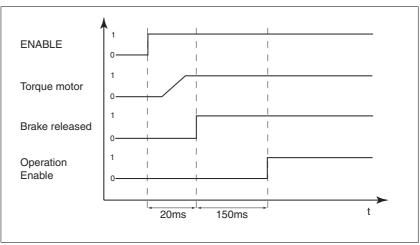
Figure 8.29 Releasing the holding brake
