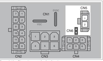
Figure 6.13 Pin assignment of safety function
