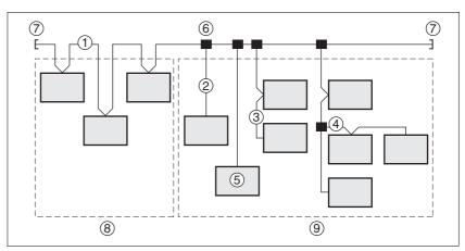
Figure 4.1 A possible DeviceNet structure
