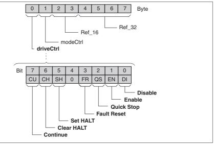
Figure 8.3 Structure of driveCtrl
