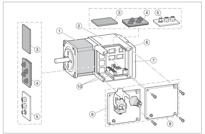
Figure 1.2 Components and interfaces
