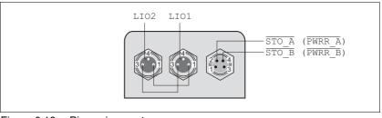
Figure 6.19 Pin assignment
