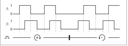
Figure 6.16 AB encoder signals
