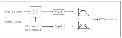
Figure 8.11 Operating mode Profile Velocity, effects of adjustable parameters
