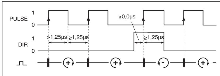
Figure 6.15 Pulse/direction signals
