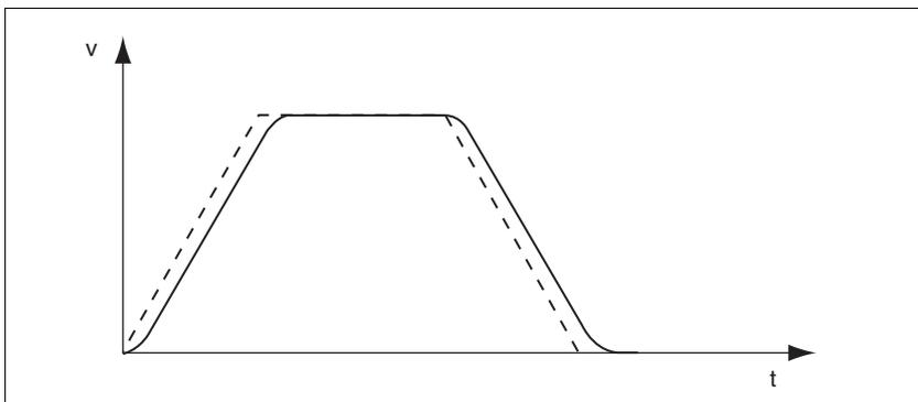
Figure 8.28 Speed curve with and without (dotted) jerk limitation
