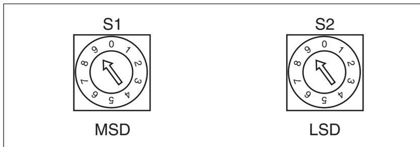
Figure 7.1 Factory settings of the rotary switches
