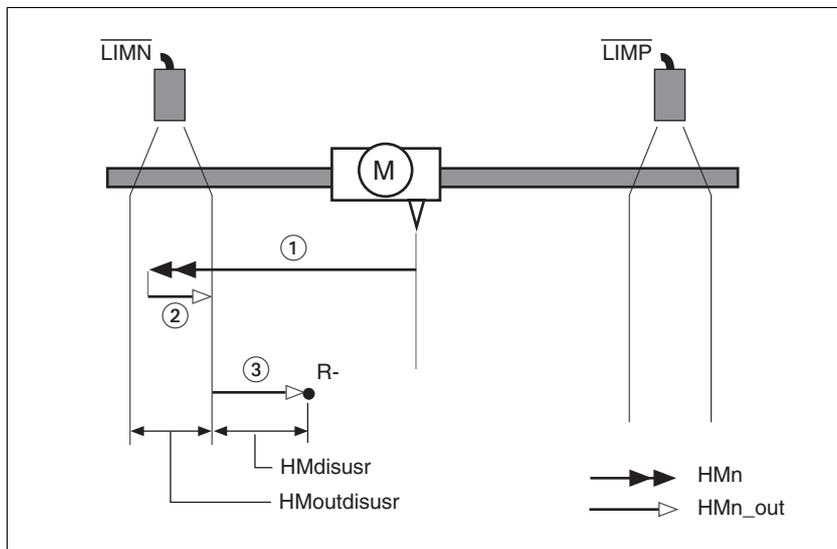
Figure 8.12 Reference movement to the negative limit switch
