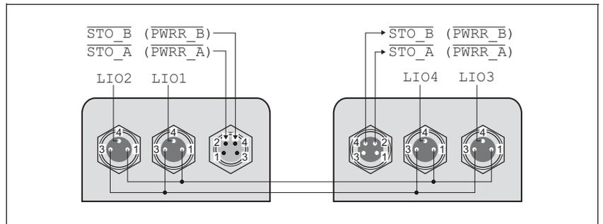
Figure 6.21 Pin assignment
