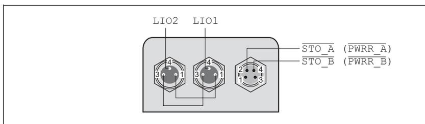
Figure 6.19 Pin assignment
