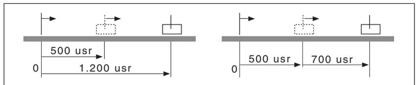
Figure 8.9 Absolute positioning (left) and relative positioning (right)
