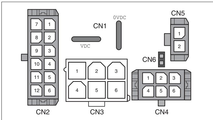
Figure 3.4 Overview of printed circuit board connectors
