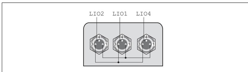
Figure 6.18 Pin assignment
