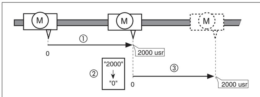
Figure 8.19 Positioning by 4000 usr units with position setting
