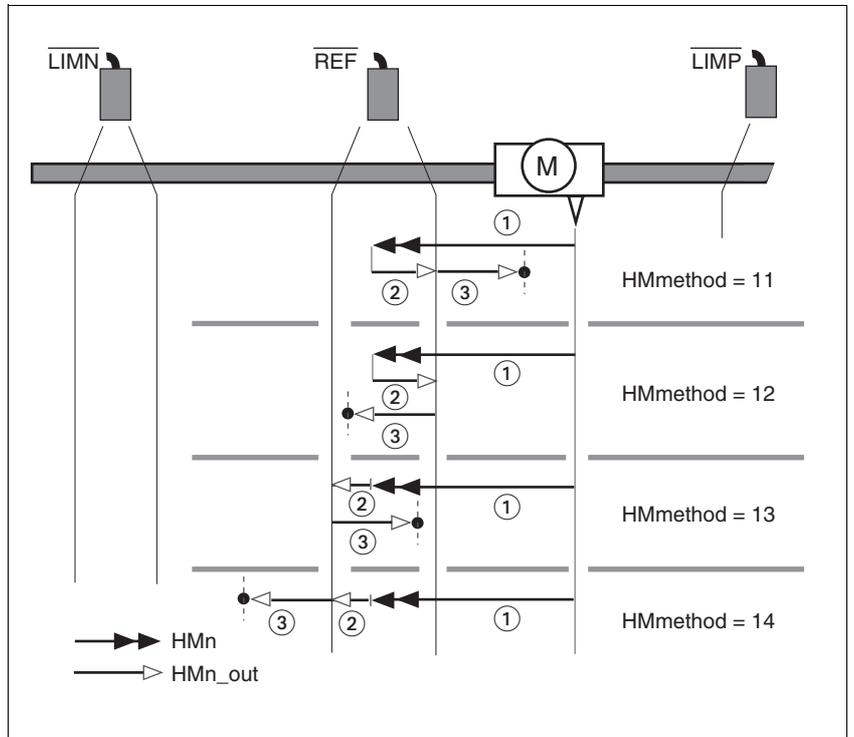
Figure 8.16 Reference movements to the reference switch
