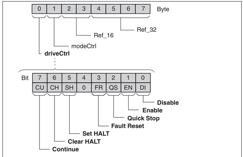
Figure 8.3 Structure of driveCtrl
