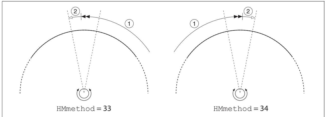
Figure 8.18 Reference movements to the index pulse
