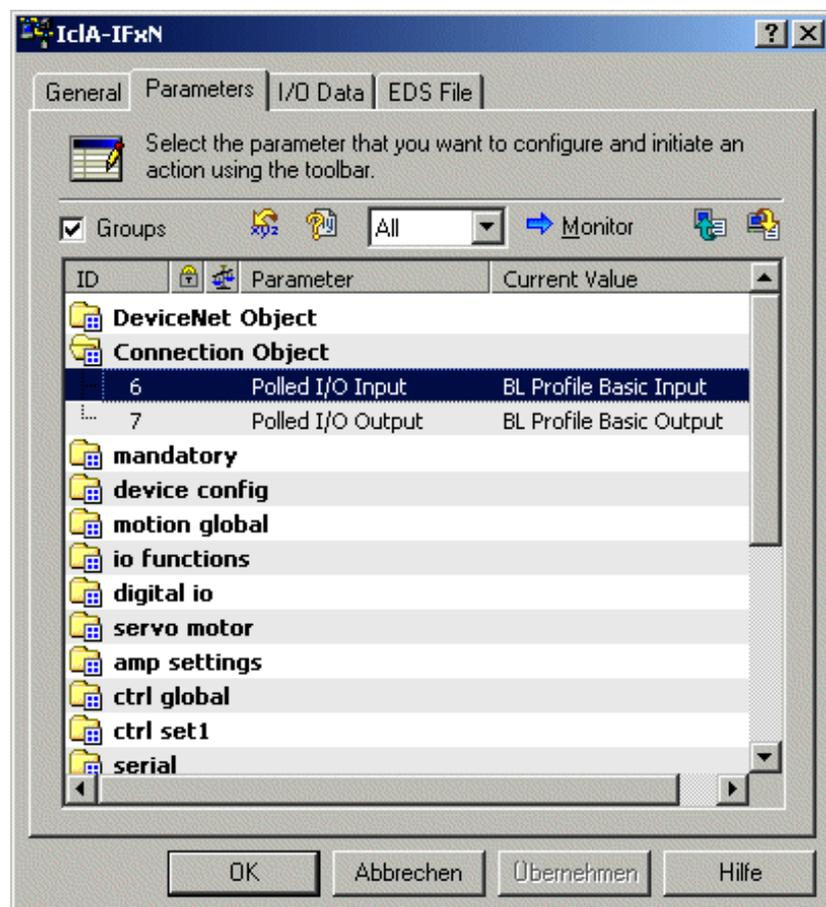
Figure 7.2 Configuring the Connection Object in the device
