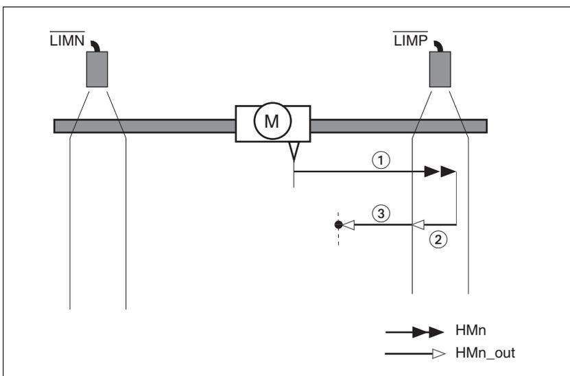
Figure 8.15 Reference movement to the positive limit switch
