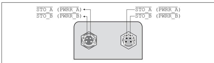
Figure 6.20 Pin assignment
