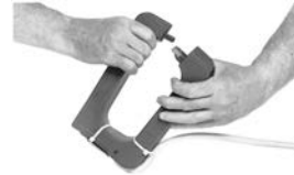
Twisting motion opens to CT diameter of round CT and smaller distance of rectangular CT. NOTE: Open split-core with a twisting motion only.
