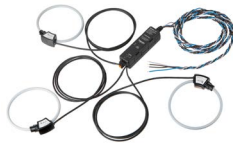
EM4200 System Calibrated with Calibrated Rogowski Coils
