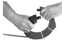
Twisting motion opens to CT diameter of round CT and smaller distance of rectangular CT. NOTE: Open split-core with a twisting motion only.
