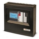
The fire panel controls the fire detection and extinguishing system. The panel can monitor two distinct areas, can trigger at least 2 levels of alarms, and incorporate a delay to evacuate the room before activating the extinguishing system. The system can also be activated by a manual switch attached to the panel.
