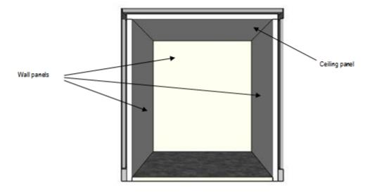
Panels will be installed on the walls and ceiling and will be composed of a sandwich of materials with fire resistance and thermal insulation to resist high temperatures and provide a watertight enclosure. The sandwich will be covered by one layer of galvanized steel sheet (0,6 mm) which will be joined by continuous weld panel to panel.
