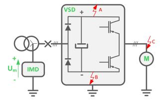
Advanced IMDs are using AC measurement voltage, either low frequency or multi frequency voltage and are compliant with DC power systems and AC/DC power systems.
