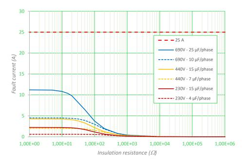
Fault current as a function of the insulation resistance
