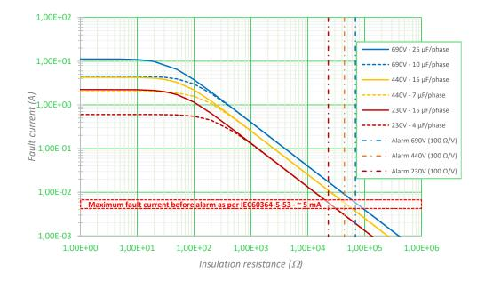
Even under humid conditions, **Figure 4** demonstrates that low insulation doesn't create dangerous touch voltages considering typical leakage capacity values as per **Table 1**.
