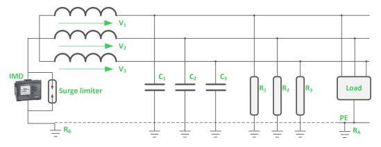
The surge limiter (**Figure 10**) prevents against damages caused by over-voltages due to internal disruptive breakdown between the MV/LV windings of the transformers or in case of lightning overvoltage.
