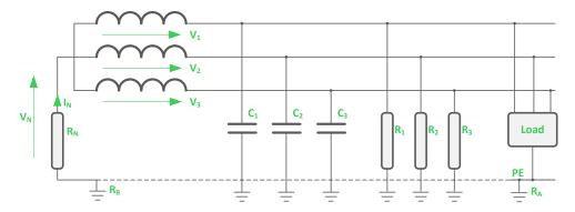
• In normal situation (no earth fault, Figure 2), currents through insulation resistances and capacitances are balanced thus  $\sum I_{ci} = \sum I_{Ri} = I_N = 0$  and there no hazardous voltage between load case and earth (Uc = 0 V).
