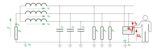
Due to their high value compared to capacitance at 50 or 60 Hz, the leakage resistances impact on the fault current IF can be neglected.
