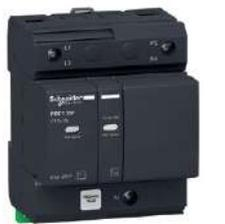
Certified for short-circuit current withstand,  $I_{sc}$  up to 75 kA (IEC 61643-11:2011). Acti9 iPRD1 F25r surge arrester version is a self-protected solution with integrated back-up Fuse (easy selection and installation). All others must be associated with an upstream fuse or circuit-breaker.
