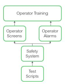
These same tests can also be used to aid the plant operators and gain valuable experience in a simulated environment. For example, test scenarios can be built for start-up, shutdown and abnormal operating conditions. Test scripts and scenarios can be used to test operating procedures. Operator performance can be measured on benchmarked including response times / reaction times under simulated abnormal operating conditions.
