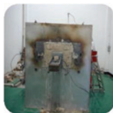
Fire resistance in building penetration
