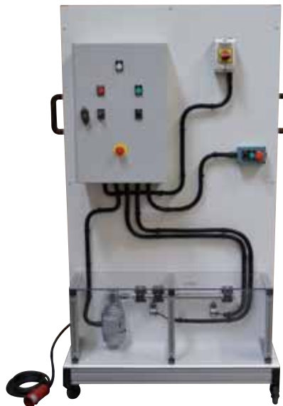
Wired accreditation test bench with motor and ball screw
