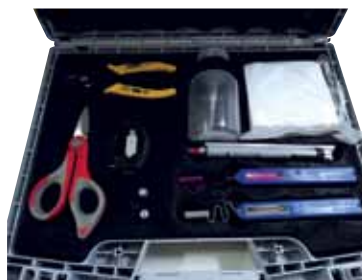
Fibre optic service case
