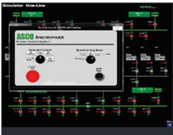
Generator Controls Station
