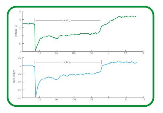
Figure 6 Battery cranking voltage signals (source: Grube
