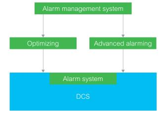
The alarm system of the DCS is the executer of all alarm functions. However, the alarm management system is the monitor and optimizer for the DCS alarm system, which is used to reduce nuisance alarms, rationalize related alarms, avoid alarm floods, and so on. In addition, some advanced alarm functions, like alarm shelving and alarm suppression, can be added to the existing DCS alarm system to make it more effective.
